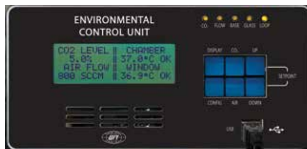
The Environmental Control Unit home screen shows the real time readings for the parameters you want to see.
