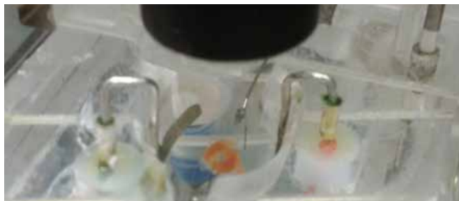
The SI-BF-100 Organ/tissue bath setup with an SMA single emission probe for direct sensing of calcium fluorescence signal. Photo courtesy of Professor Andreas Dendorfer, Walter Brendel Zentrum, München, Germany.
